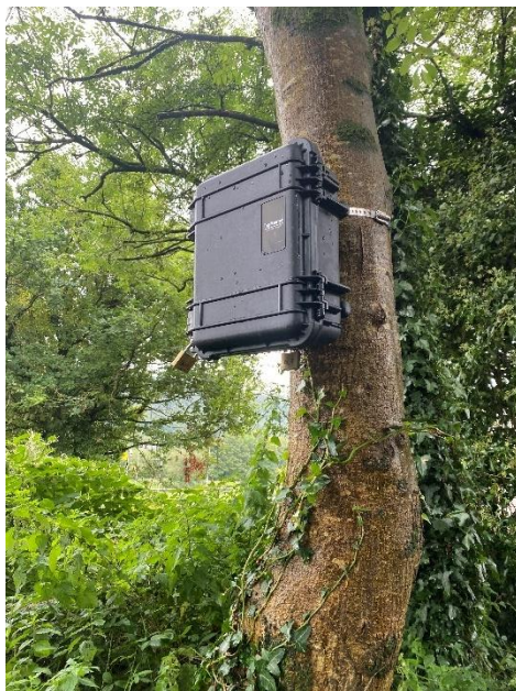
Figure 7: Picture of a radar box capturing walking and cycling data on NCN43.
