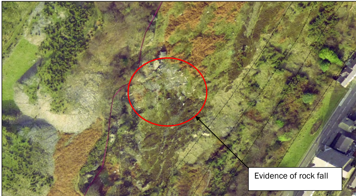
Insert 43 - Rock fall from the former quarry face/back scar
