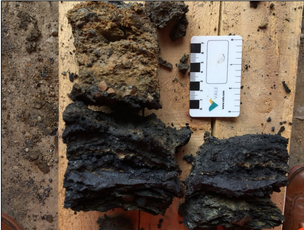
Insert 31 - Silty clay infill in BH602. Interpreted as a shear surface.
