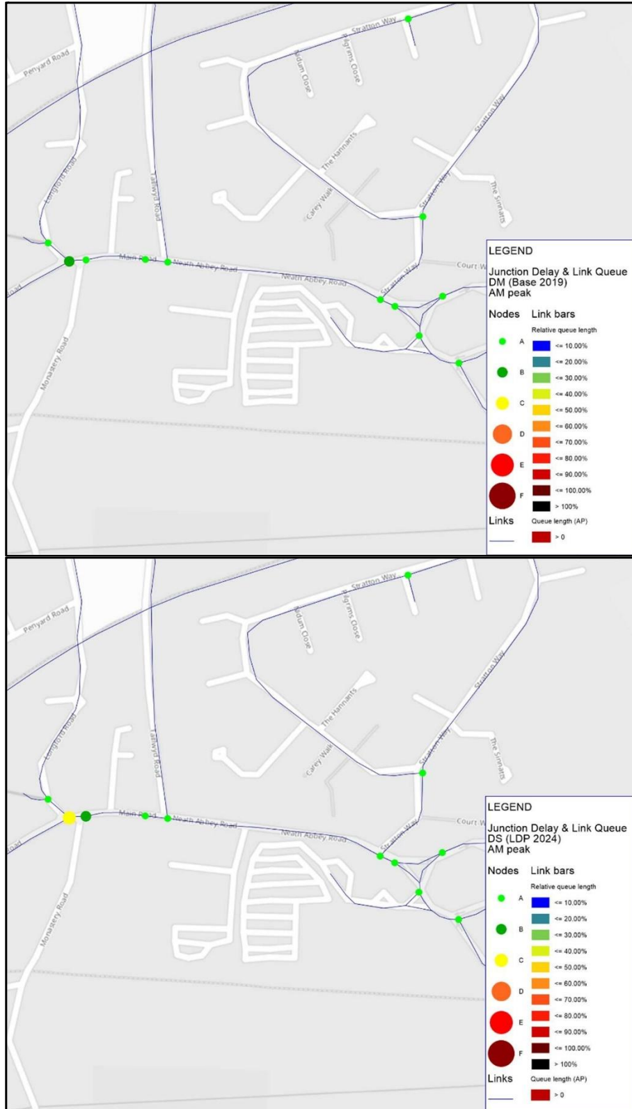
Figure 8: - Junction delay and link queues: AM A4320 towards Tesco roundabout (Base 2019 top, LDP 2024 bottom)
