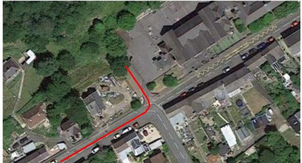
Proposed access route 2 along Cilmaengwyn/Graig Road and up the widened primary school car park access road. This access will be utilised to remove any tip material that can't be transported up to route 1. The primary school car park will be used for turning and stacking lorries ready for loading to ensure the highway is kept clear.
